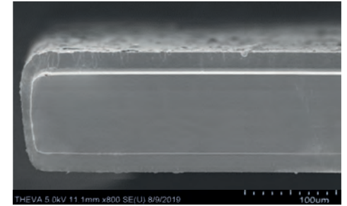
SEM cross section of PVD copper coating
