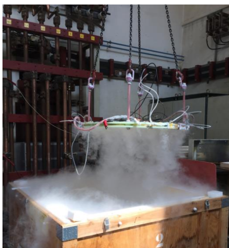
Figure 2: One pancake-shaped coil tested at IPH in Berlin.
