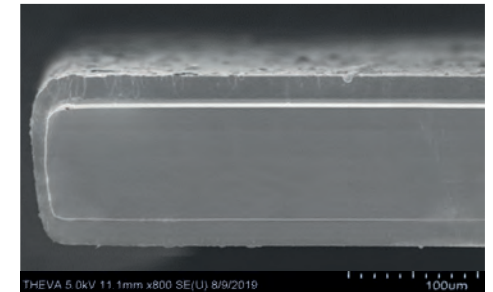
SEM cross section of PVD copper coating
